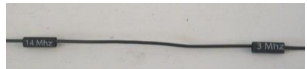
Frequency marker on the Kevlar wire
