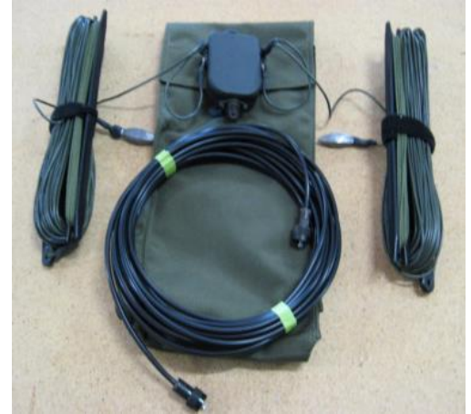
Tactical Tuned Dipole unpacked with coax Cable
